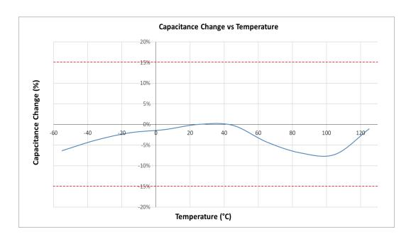
The upper and lower limit lines denote the boundaries of X7R specification (±15% from -55°C to +125°C)
